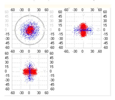
The efficiency is very bad, around 7E-9, due to a weak number of fusions and a not negligible loss of electrons, due mostly to collisions on the injector.
